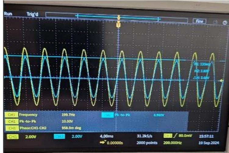
(4) Before we moved to the next part, we compared both our measurements to our calculated results from part I Step(3a). Which we should be in a reasonable agreement of 10% max error in both the real and imaginary parts.
