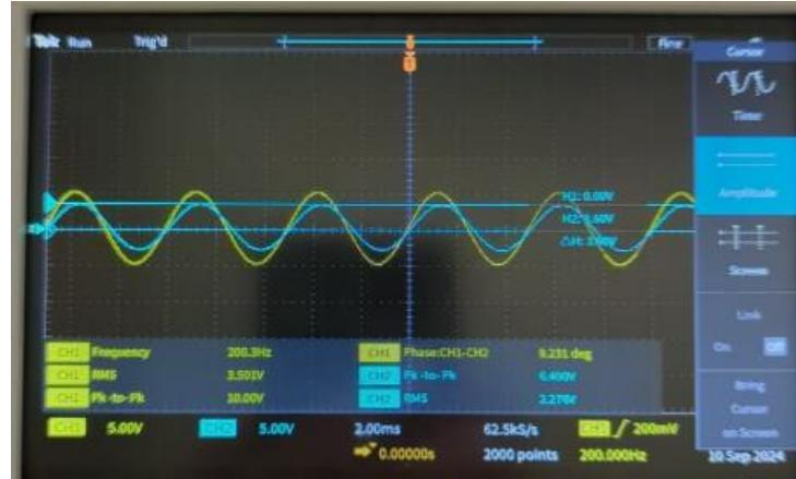
(2) We made our phasor measurements and used them to calculate the complex power. We also found real power, reactive power, apparent power, and power factor.
